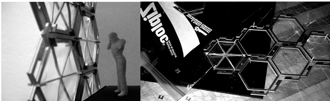
Figure 19. Waterjet cut model of System II with plastic cushions representing ETFE
