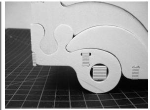
separate hinge detail: increases cutsheet efficiency eases assembly sequencing
