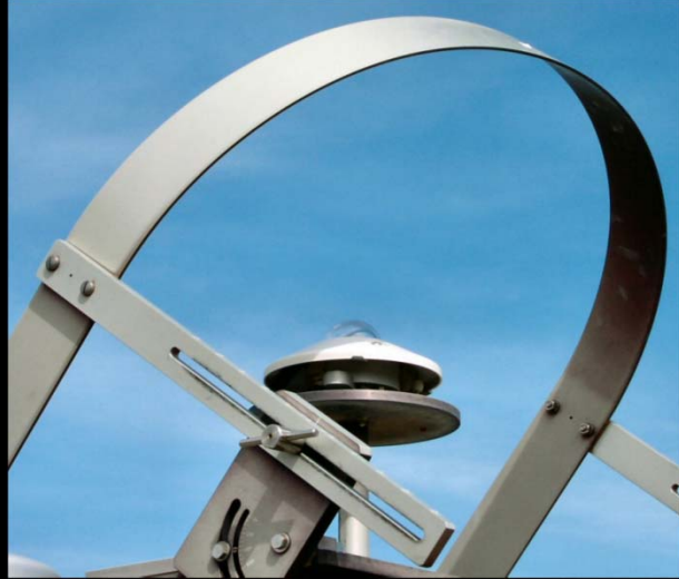
Source: Quaschnig, Volker. "Pyranometer with Shadowband." http://www.volker-quaschnig.de .
