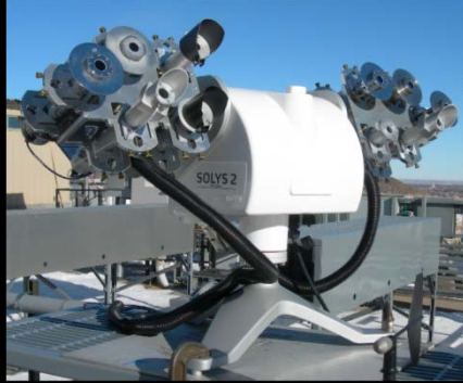
Radiometers installed on an automatic solar tracker (Photo Tom Stoffel, NREL)
