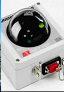
BF3 Sunshine Sensor Courtesy of Delta-T Devices Ltd. Used with permission.
