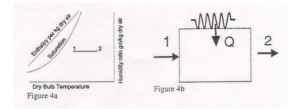
In this process, we will write the mass flow rate of dry air without the subscript a. There isn't any water vapor added to the air so the mass balance for the water becomes,
