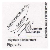
If we want to make sure the room falls within the comfort conditions, then state 1 must be located so that the line 1-2 passes through the range of comfort on the psychrometric diagram. For example, Figure 8c shows a typical condition line and summer comfort zone. With the original state of inlet air to the space, labeled 1, the condition line does not pass through the comfort zone no matter what airflow rate is used. The inlet air must be altered to state 1' to achieve comfortable conditions.
