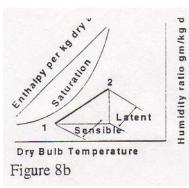
We can see that the airflow rate into the room falls out and the ratio of  $\Delta\omega/\Delta h$  is determined by the ratio of latent to total energy input. That is, the state of the well mixed air in the room, state 2, must be on the line, called the condition line, with slope  $\Delta\omega/\Delta h$  which passes through the inlet state 1 as shown on Figure 8b.
