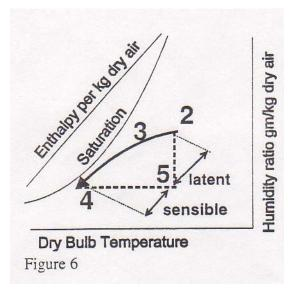
In theory the process from state 2-3-4 could be replaced first by a reduction in water vapor at constant dry bulb temperature, process 2-5, Figure 6, followed by a reduction in dry bulb temperature at constant water vapor content, process 5-4. The latter process is one of pure sensible heat,
