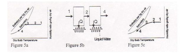
2 since  $\omega$  remains constant. Note that the relative humidity decreases in this process as the dry bulb temperature increases.
