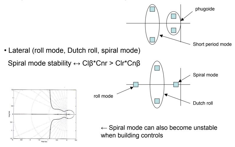
effects on stability of a loop of  $\Phi$  on  $\delta a$
