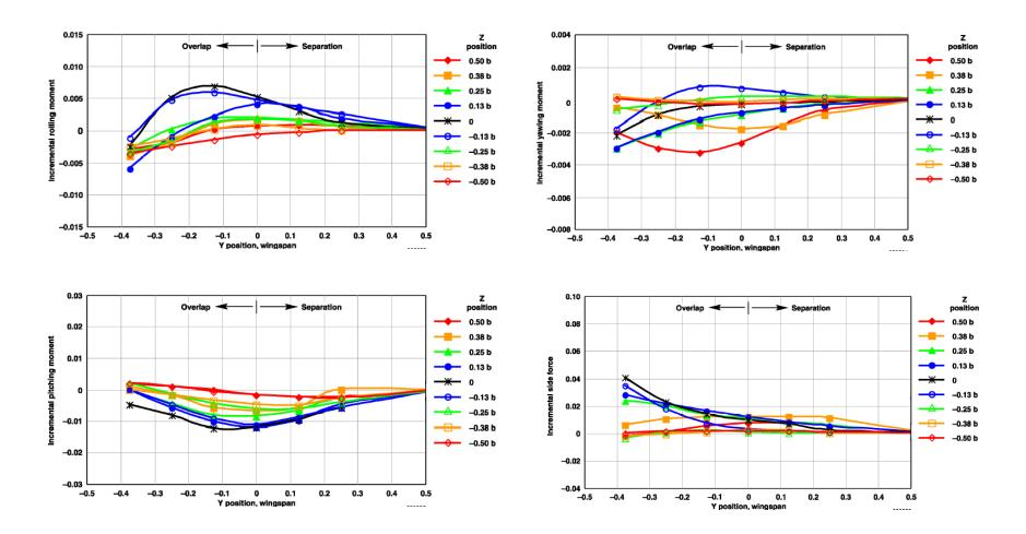
Vortex effects are weaker at transonic than at subsonic conditions
