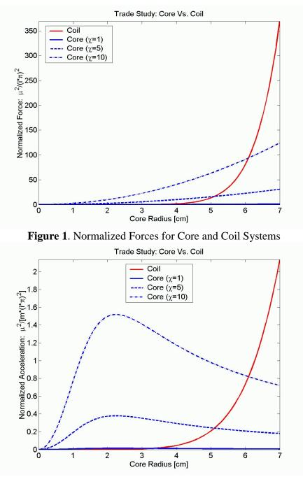
Figure 2. Normalized Accelerations for Core and Coil Systems
