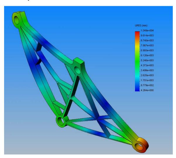
Figure 1: Mode Shape 1 @ 460 Hz of Version 1 for Team 5
