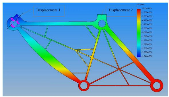
Figure 5: Displacement in the X direction in mm
