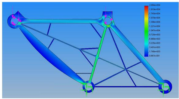
Figure 3: Von Mises Stress plot
