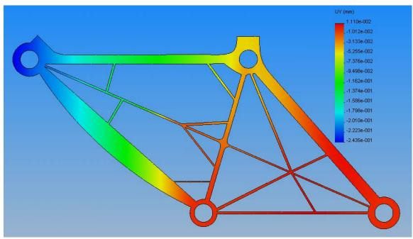
Figure 4: Displacement in the Y direction in mm
