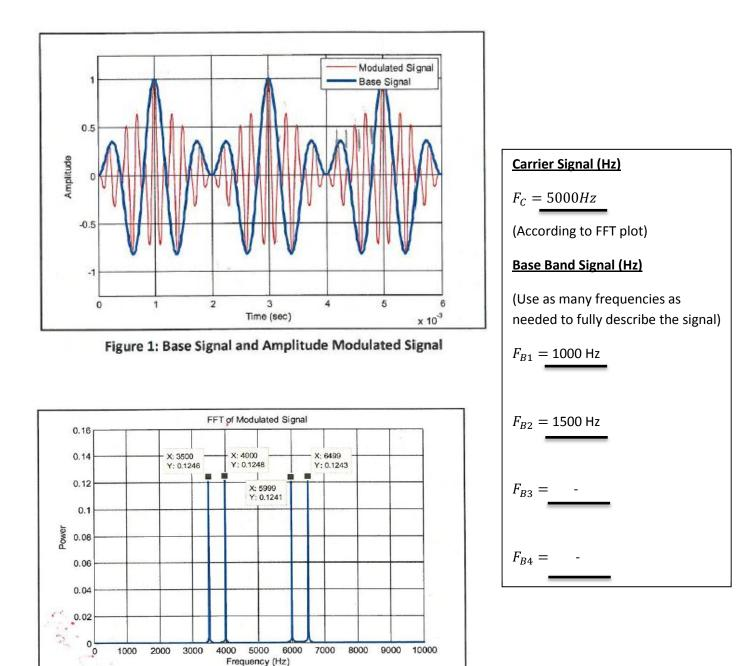
Figure 2: FFT of DSB-SC Signal (Positive Transform Only)
