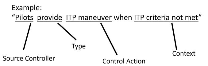
Four parts of a hazardous control action
