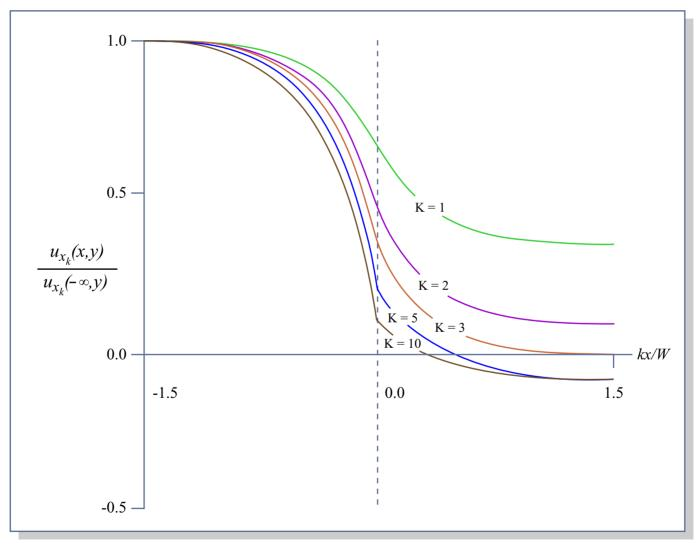
A MORE COMPLICATED (OR IS IT?) EXAMPLE: STATIC PRESSURE FIELD UPSTREAM OF A COMPRESSOR STATOR/STRUT GEOMETRY [The figure shows only one section (one "wavelength") of a periodic geometry]
