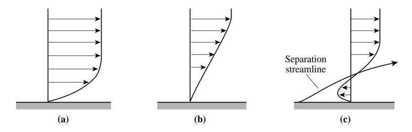
• The ∆*p* at which ∆*u* is driven to 0 in BL is less than that which freestream can attain
