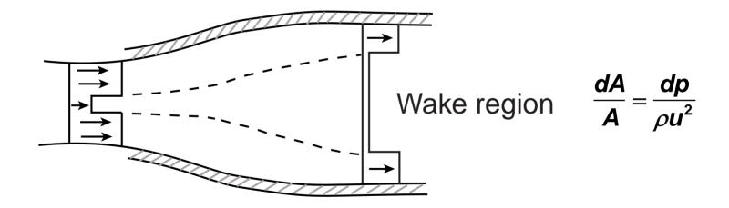
• In a favorable pressure gradient the wake (or boundary layer) is accelerated more and "thins out"
