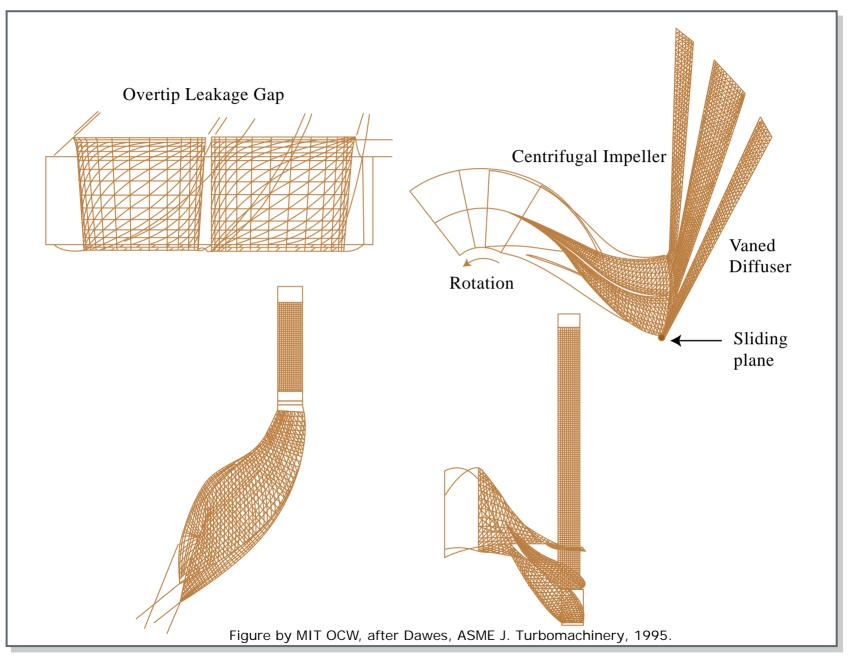
Figure 6: Unstructured mesh generated for the splittered impeller.
