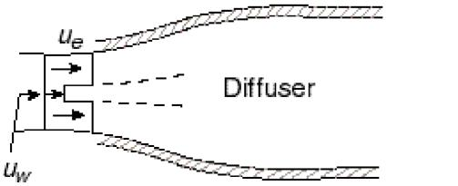
Locally,  $\frac{dp}{\rho u} = -du$  is pressure rise (drop) velocity relation dp is same for wake and freestream u is lower in the wake  $|du_{wake}| > |du_{wake}|$
