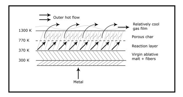
For the shuttle RSRM, the throat insert (C cloth phenolic) regresses ~ 1 inch/120 sec, and the char depth is ~  $0.5^{\circ}$  inch/120 s.
