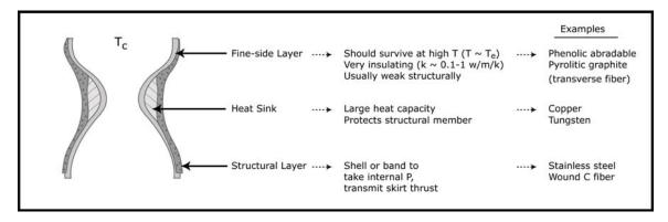
Inner layer retards heat flux to the heat sink. Heat sink's T gradually rises during firing (60-200 sec). Peak T of heat sink to remain below matl. limit. Back T of heat sink to remain below weakening point for structure.
