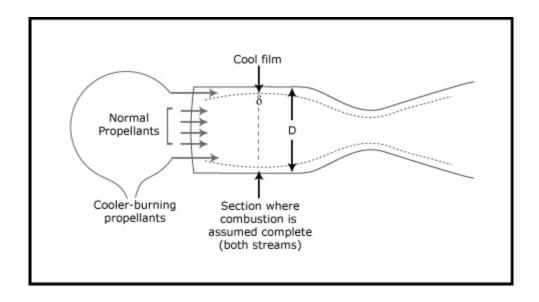
For application of data on slot-injected films, we need to define the initial film thickness s, velocity  $u_{_{\! F}}$  , density  $\rho_{_{\! F}}$  , or at least mass flux  $u_{_{\! F}}\rho_{_{\! F}}$  .
