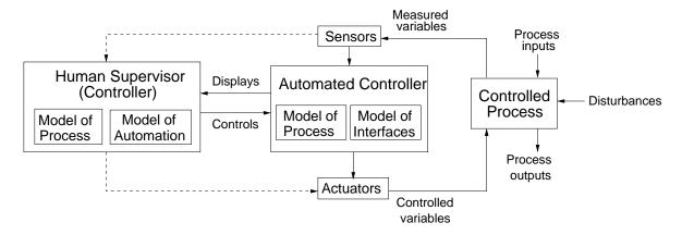
Figure 1: A standard control loop.
