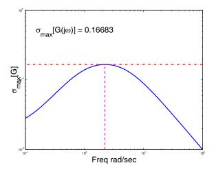
Figure 15.1: Graphical test for the  $||G||_{\infty}$ .
