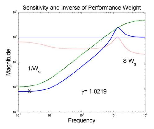
Fig. 2: Want  $|SW_p| < 1$ , so we just fail the test
