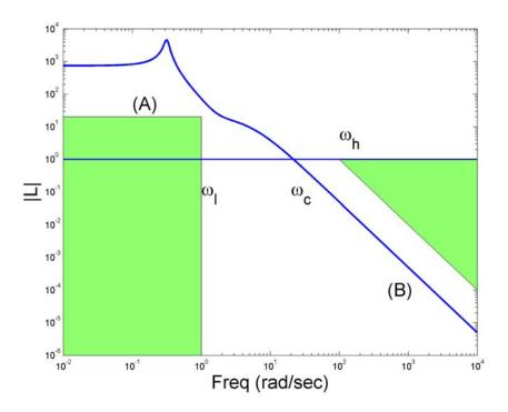
(A) High loop gain → Good command following & dist rejection
