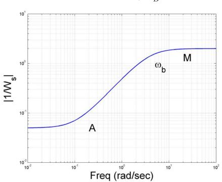
Fig. 1: Example of a standard performance weighting filter. Typically have  $A\ll 1$ , M>1, and  $|1/W_s|\approx 1$  at  $\omega_B$
