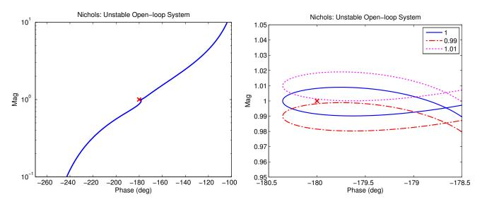
Fig. 4: Nichols Plot ( $|L((j\omega))|$  vs.  $\arg L((j\omega))$ ) for the cart example which clearly shows sensitivity to overall gain and/or phase lag.
