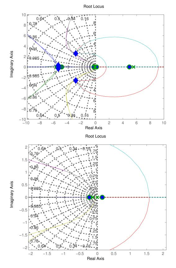
Fig. 3: Root Locus with frozen compensator dynamics. Shows sensitivity to overall gain – symbols are a gain of [0.995:.0001:1.005].
