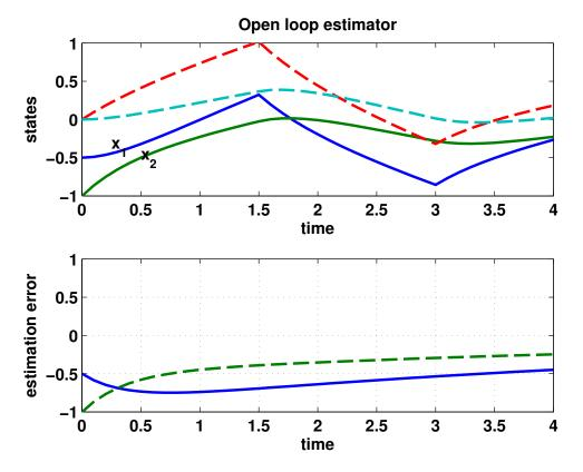
Fig. 1: Open-loop estimator error converges to zero, but very slowly.
