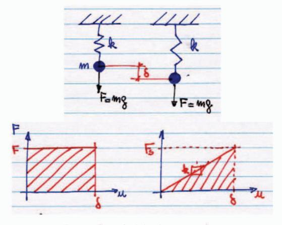
Figure 2: Spring loaded with a constant force
