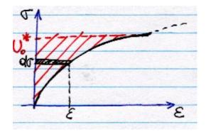
Figure 4: Complementary strain energy density
