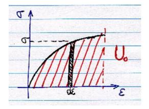
Figure 3: Strain energy density
