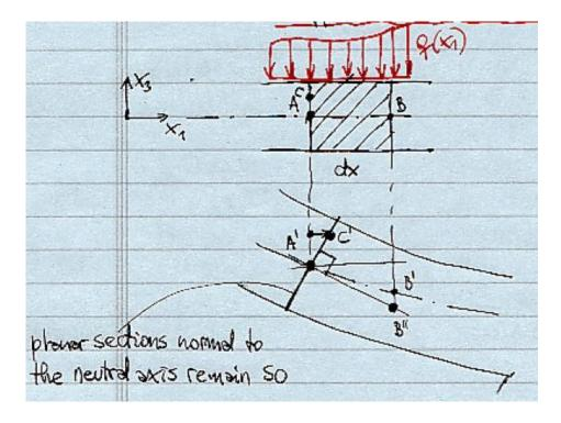
Figure 1: Kinematic assumptions for a beam
