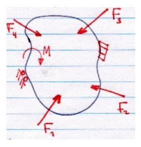
Given a body in equilibrium under the action of N concentrated forces  $F_I$ . The potential energy of the external forces is given by:
