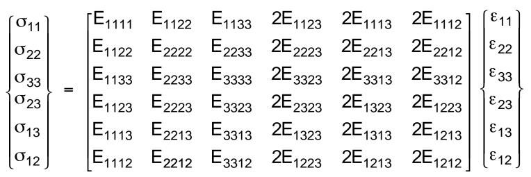
Results in 21 independent components of the elasticity tensor
