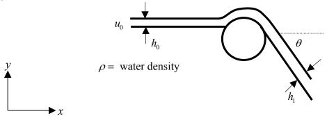
Consider a stream of water with initial velocity  $u_0$  and width  $h_0$  which impinges on a cylinder of radius *R* as shown in the figure. The stream eventually separates from the cylinder at an angle  $\theta$  and width  $h_1$ . Using the integral conservation equations, calculate the force in the x and y directions of the water acting on the cylinder? Assume the cylinder is fixed.
