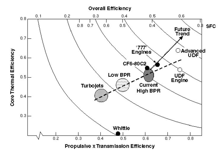
Trends in *thermal efficiency* are driven by increasing compression ratios and corresponding increases in turbine inlet temperature. Whereas trends in *propulsive efficiency* are due to generally higher bypass ratio engines
