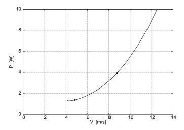
Figure 2: Thrust power P = DV for electric sport aircraft.
