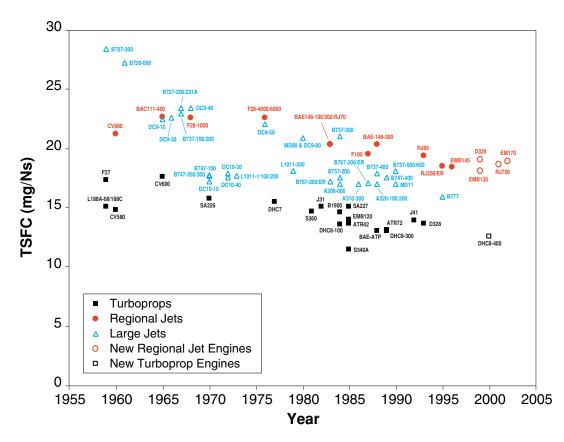
**Figure 1.9** Engine efficiency for commercial aircraft: specific fuel consumption (Babikian, R., *The Historical Fuel Efficiency Characteristics of Regional Aircraft From Technological, Operational, and Cost Perspectives*, SM Thesis, MIT, June 2001)
