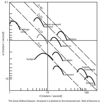
The Great Gliding Diagram. Airspeed, V, is plotted on the horizontal axis. Rate of descent, w, is plotted downward along the vertical axis. The diagonals are lines of constant finesse. The horizontal line represents the practical soaring limit, 1 meter / second.
