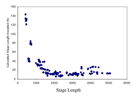
**Figure 1.11** Deviation (%) of Breguet range equation estimates from actual stage length flown is a function of the stage length (J. J. Lee, MIT Masters Thesis, 2000)
