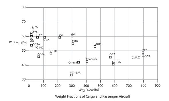
Figure 1.5 Weight fractions for transport aircraft in terms of empty weight over max take-off weight (Mattingly, Heiser & Daley, <u>Aircraft Engine Design</u>, 1987)
