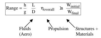
Note that this expression is sometimes rewritten in terms of an alternate measure of efficiency, the *specific fuel consumption* or SFC. SFC is defined as the mass flow rate of fuel per unit of thrust (lbm/s/lbf or kg/s/N). In the following expression, V is the flight velocity and g is the acceleration of gravity.
