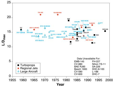
Figure 1.4 Aerodynamic data for commercial aircraft: L/D for cruise (Babikian, R., *The Historical Fuel Efficiency Characteristics of Regional Aircraft From Technological, Operational, and Cost Perspectives,* SM Thesis, MIT, June 2001)
