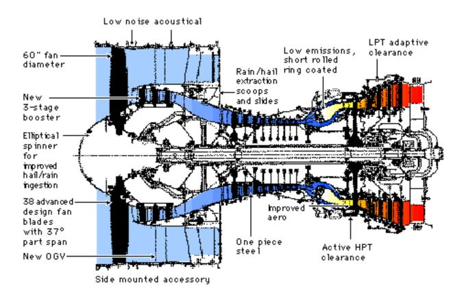
Measure the inlet and exit blade angles near the root of the fan and the inlet blade angle of the first stator blade on the 3-stage low pressure compressor (the "booster" as labeled above).
